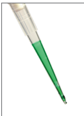
Conventional tip after dispensing 100 µL sample.
