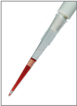
Liquid passes through conventional filter pipet tips causing cross contamination.
