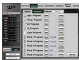
Control / Manual - Performs manual, sequence or EZ Script control(optional) of each parameter.
