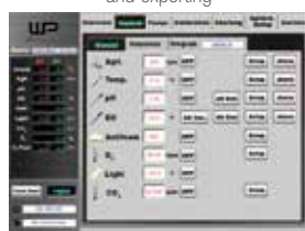
Control / Manual - Performs manual, sequence or EZ Script control(optional) of each parameter.
